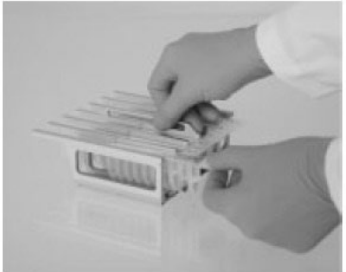
Figure 3. Ease of setup using reagent cartridges. (A) A sealed, prefilled reagent cartridge. Fill levels vary, depending on the type of reagent cartridge. (B) Loading reagent cartridges into the cartridge rack. The cartridge rack itself is labeled with an arrow to indicate the direction in which reagent cartridges must be loaded.
