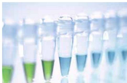
Figure 2. Built-in pipetting control. The QuantiNova Probe PCR master mix contains an inert blue dye that turns green on addition of the template nucleic acid diluted in the yellow nucleic acid dilution buffer, providing a visual indication of correct pipetting.
