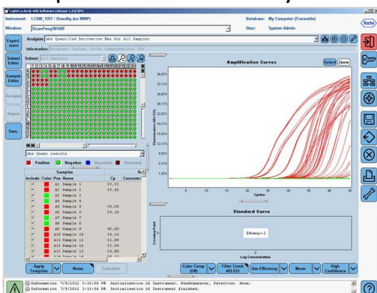
Figure 9. Obtaining the crossing point (Cp) cycle values at the second derivative maximum.
