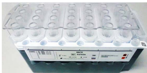
Reagent cartridge in reagent cartridge holder with enzyme rack and piercing lid.
