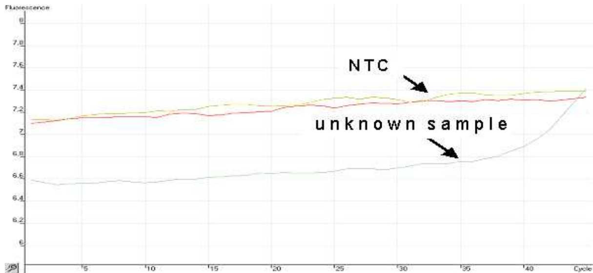
Figure 6: Single amplification curve analysis (SACA) of a sample with the artus HBV RG PCR Kit using an artus 3000 Instrument. The amplification curves of an unknown sample and those of the negative controls (NTC) are depicted. In order to increase the resolution of the presentation, the raw data (Raw Channel) were analyzed and the scaling of the depiction was automatically carried out (Auto-Scale). The comparison between the shape of the amplification curve of the sample and those of the negative controls allows an assessment (positive or negative) of the unknown sample. After this analysis the PCR of this unknown sample may be assessed as low positive.
