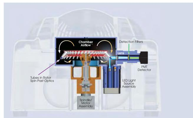
**Figure 1. Cross-section of the Rotor-Gene Q.** Heating/cooling is achieved by rapid airflow in the reaction chamber. Tubes spin past the excitation/detection optics every 150 milliseconds enabling high-speed data capture. Up to 6 separate LED light sources can be used in combination with 6 different detection filters and a highly sensitive photomultiplier detector.
