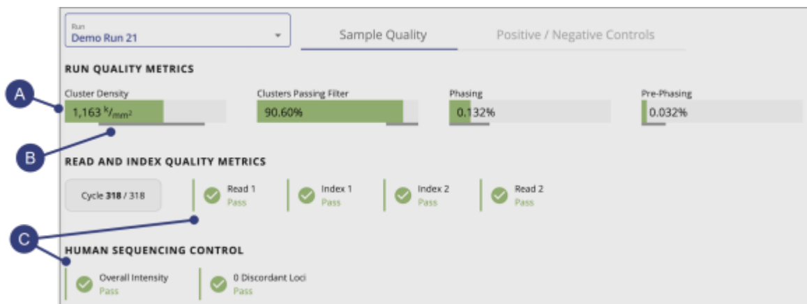
Figure 6. Quality metrics overview. [A] Color-coded horizontal bars and values indicate run quality metrics. [B] Thinner horizontal bars in dark gray indicate optimum ranges. [C] Color-coded vertical bars and icons indicate the quality of each read and the HSC.
