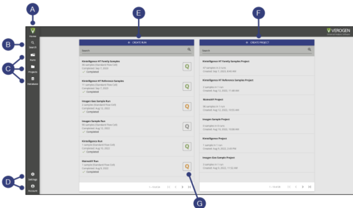
Figure 1. Overview of the Home page. [A] Navigation rail — Buttons to open workspaces, search for a sample, run, or project, access settings, or return to the Home page. [B] Search — Search for a sample, run, or project by name or date. [C] Workspaces — Open one of the primary workspaces. [D] Settings — Access software or account settings. [E] Runs — A list of the most recent runs, with options to create a new run or search for an existing run. [F] Projects — A list of the most recent projects, with options to create a new project or search for an existing project. [G] Quality Metrics icon—This icon displays color-coded quality metrics for a completed run; hovering over it reveals detailed metrics.
