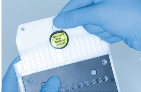
Figure 6. Preparing the QIAxcel Gel Cartridge.
