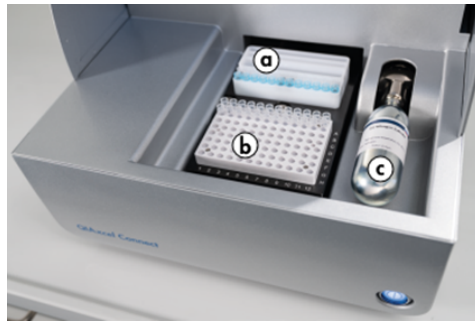
Figure 4. Buffer tray holder (a), sample plate holder (b), and N2 port (c) location.
