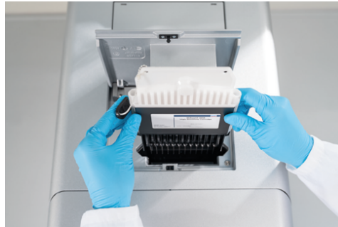
Figure 9. Installation of QIAxcel Gel Cartridge.
