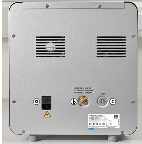
Figure 5. Power connection (a), external N2 (b), and USB port (c).
