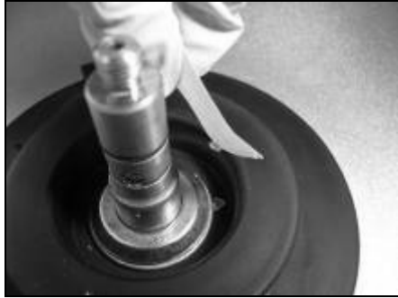
Removing plastic debris with tape.
