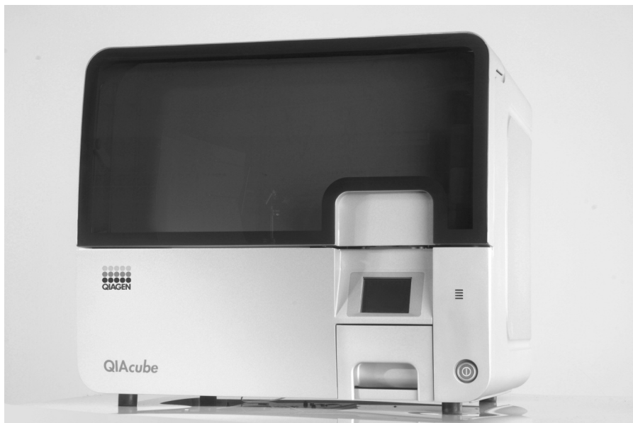
Figure 1. Automated DNA purification. DNA purification using the QIAamp DNA Stool Mini Kit can be automated on the QIAcube.
