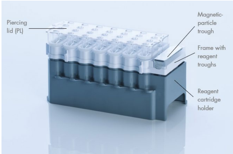
Figure 2. QIASymphony reagent cartridge. The reagent cartridge contains all reagents required for the protocol run.
