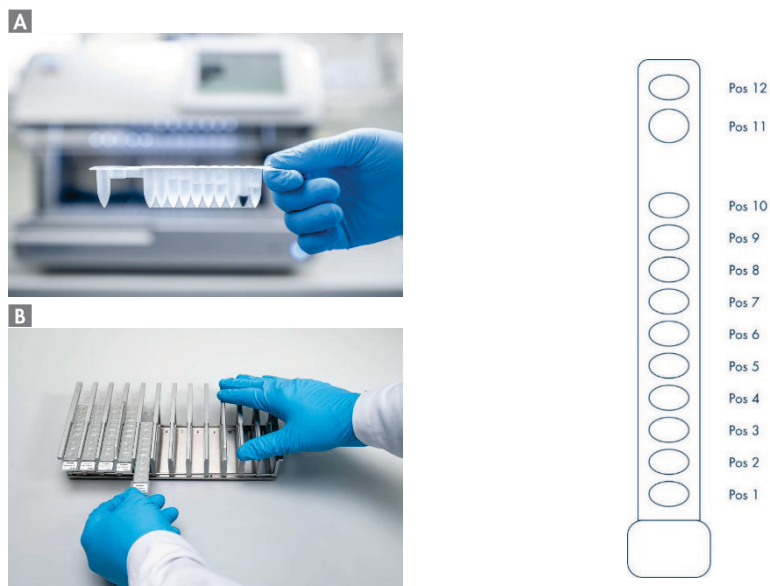
Figure 2. Ease of worktable setup using reagent cartridges. (A) A sealed, prefilled reagent cartridge. Fill levels vary, depending on the type of reagent cartridge. (B) Loading reagent cartridges into the cartridge rack. The cartridge rack itself is labeled with an arrow to indicate the direction in which reagent cartridges must be loaded. Each reagent cartridge contains 12 individual positions.
