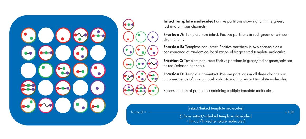
Mathematical approximations for estimation of dPCR template integrity. Schematic representation of a QIAcuity nanoplate. Partitions containing one or more intact or non-intact template molecules are shown. The template contains 3 targets addressed in a triplex reaction within the green, red and crimson channels. Not all possible fragmentation and distribution scenarios are shown. % intact represents the calculated integrity of the analyte of interest.
