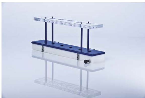
Figure 1. Basic Carrier with Elution Rack in parking position.
