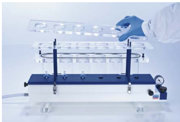
Figure 17. Removing the upper Cross-Beam from the Column Holder.
