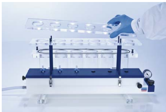
Figure 21. Replacing the upper Cross-Beam onto the Column Holder.
