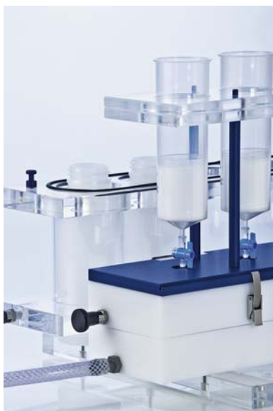
Figure 12. Collection vessels inserted into the corresponding holders of the Elution Rack in parking position.
