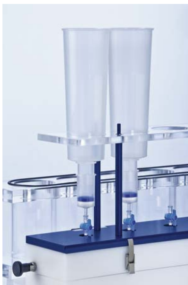
Figure 19. Set up of QIAconcentrator-Tube Extender assembly in the QIAvac HiSpeed LS.
