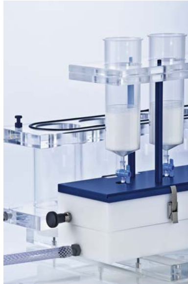
Figure 10. HiSpeed Giga-tip inserted into the luer slot of the VacValve.
