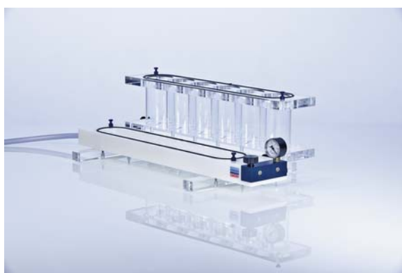
Figure 1. Basic Carrier with Elution Rack in parking position.
