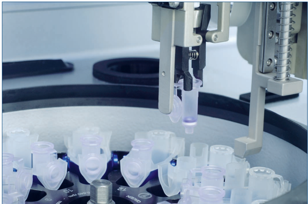
Figure 3. Freedom from laborious manual tasks. The QIAcube is equipped with an automated centrifuge and pipetting system. No manual handling steps are required.
