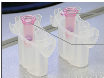
Comparing correct and incorrect removed column lids.
