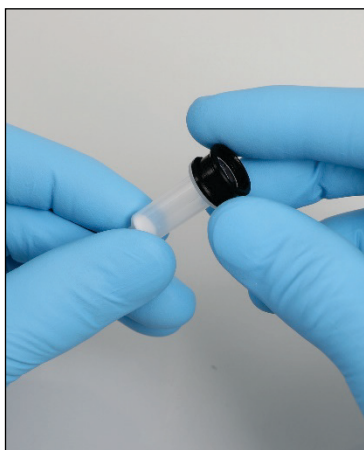
Mounting a spin column adapter ring.
