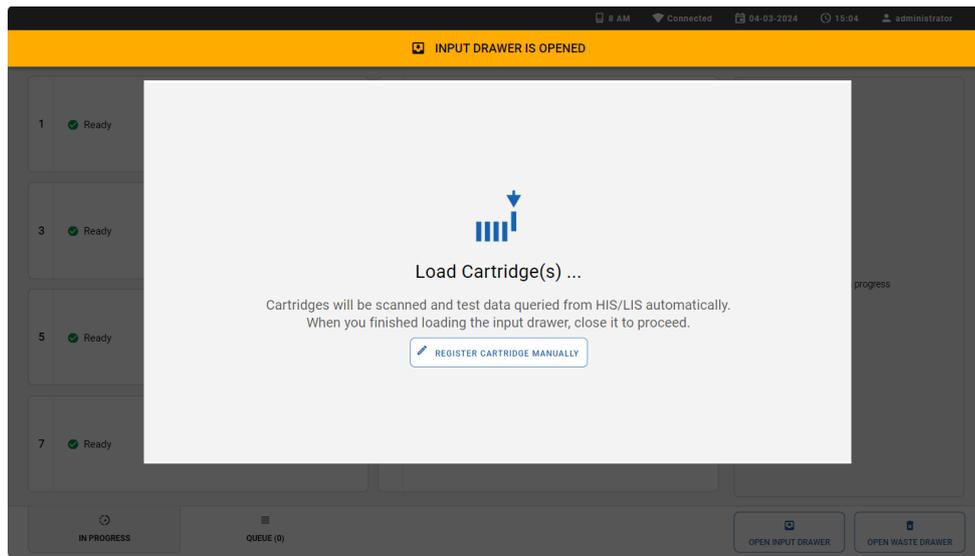
Figure 11. The load cartridge dialog when the test order functionality is enabled and force order disabled
