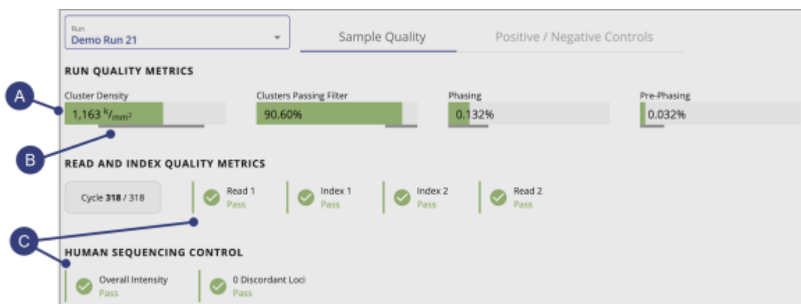
Figure 9. Quality metrics overview. A. Color-coded horizontal bars and values indicate run quality metrics. B. Thinner horizontal bars in dark gray indicate optimum ranges. C. Color-coded vertical bars and icons indicate the quality of each read and the HSC.
