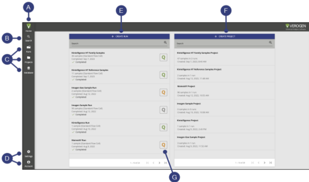
Figure 1. Overview of the Home page. A. Navigation rail — Buttons to open workspaces, search for a sample, run, or project, access settings, or return to the Home page. B. Search — Search for a sample, run, or project by name or date. C. Workspaces — Open one of the primary workspaces. D. Settings — Access software or account settings. E. Runs — A list of the most recent runs, with options to create a new run or search for an existing run. F. Projects — A list of the most recent projects, with options to create a new project or search for an existing project. G. Quality Metrics icon — Color-coded quality metrics for a completed run; hovering over the icon reveals detailed metrics.
