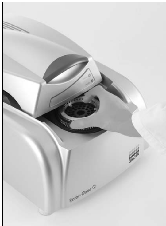
Figure 2. Transferring the samples to the Rotor-Gene Q. After sample preparation and assay setup, the reactions are loaded in the 72-Well Rotor of the Rotor-Gene Q for real-time PCR analysis.
