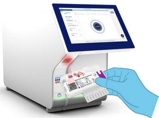
Figure 13. Scan du code-barres de la QIAstat-Dx Gastrointestinal Panel Cartridge.
