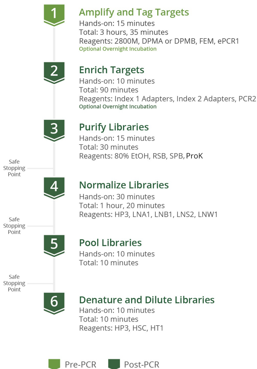
Figure 2 Overview of the ForenSeq DNA Signature Prep protocol with the ForenSeq Enhanced PCR1 Reaction Mix
