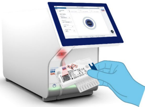
Gambar 45. Memindai barcode QIAstat-Dx Respiratory SARS-CoV-2 Panel Cartridge.
