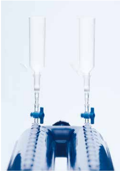
Figure 2. QIAamp Mini columns with tube extenders for processing on the QIAvac 24 Plus.
