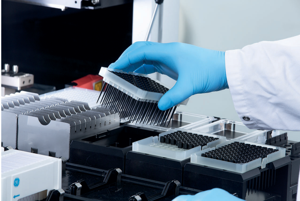
Multiflex carrier with two modules holding card recovery magazines and three tip rack modules and tip trays.
