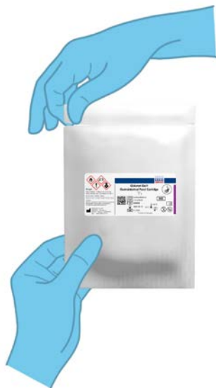
Joonis 4. Kasseti QIAstat-Dx Gastrointestinal Panel Cartridge avamine
