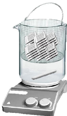
Figure 1. Beaker with tissue cassettes in a wire basket placed on magnetic stirrer for manual processing of PAXgene Tissue treated specimens.
