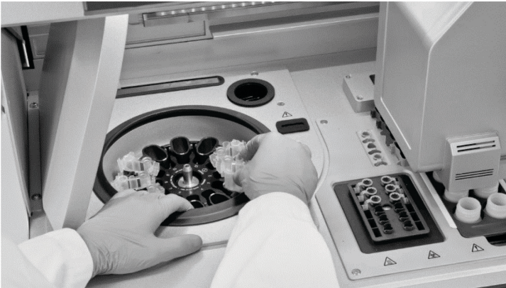
Figure 21: Loading the centrifuge on the QIAcube Connect MDx. Load the assembled rotor adapters into the centrifuge buckets.
