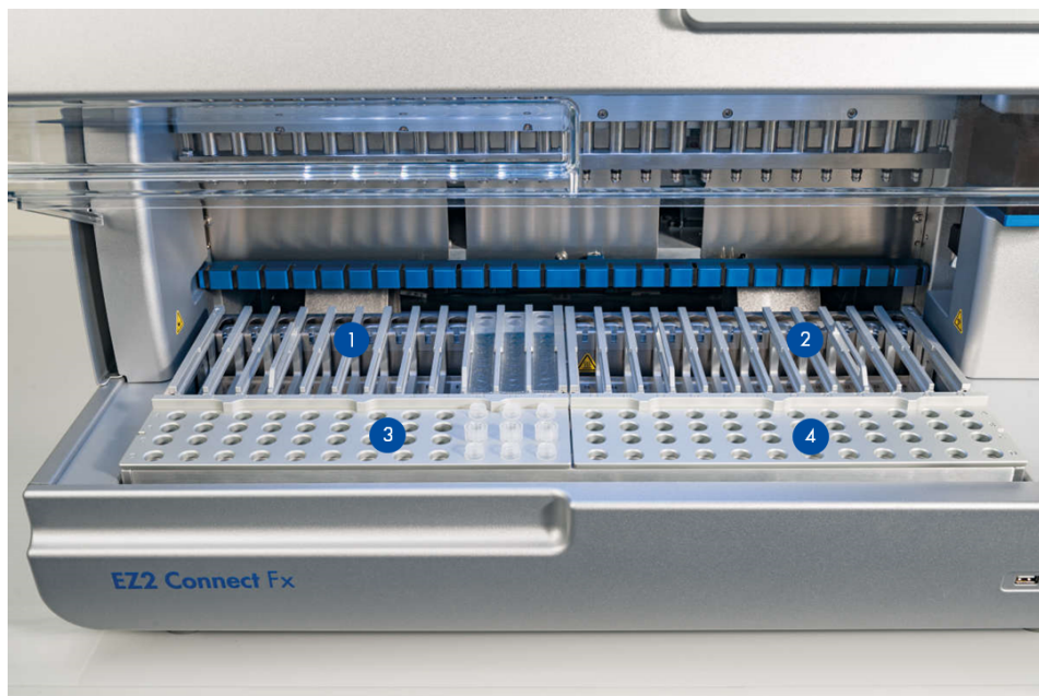
Figure 3. EZ2 Connect Fx Worktable. (1) EZ2 Connect Cartridge Rack – left. (2) EZ2 Connect Cartridge Rack – right. (3) EZ2 Connect Tip Rack – left. (4) EZ2 Connect Tip Rack – right.
