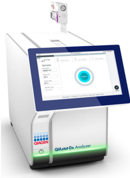
Figur 13. Sette QIAstat-Dx Gastrointestinal Panel 2 Cartridge inn i QIAstat-Dx Analyzer 1.0 eller QIAstat-Dx Analyzer 2.0.
