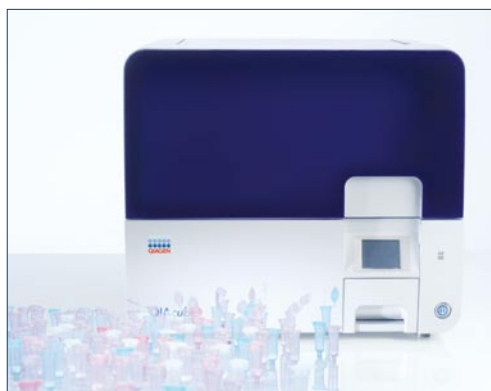
Figure 3. QIAcube. The QIAcube enables full automation of QIAGEN spin-column kits, making sample processing with the MinElute PCR Purification Kit fast and efficient.
