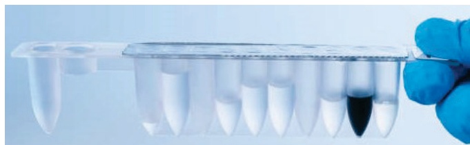
Figure 8. Reagent cartridge (RCV). A sealed, prefilled RCV of the EZ1 DSP Virus Kit.
