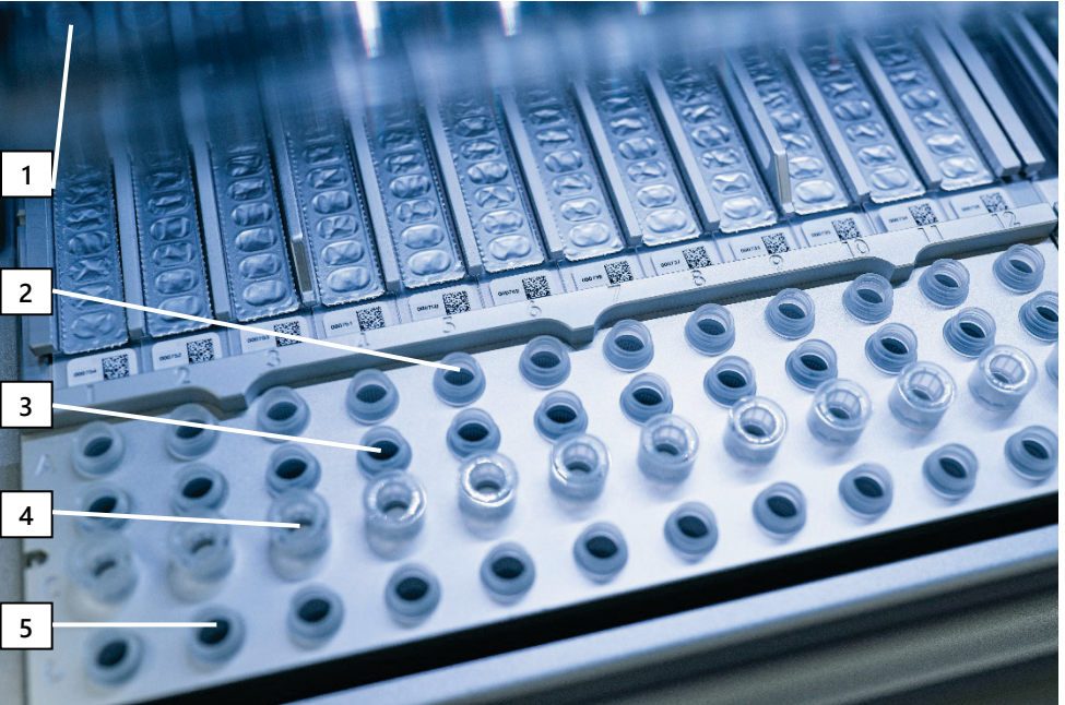
Figure 5. Worktable of an EZ2 Connect MDx instrument. (1) Heating block with 2 mL tubes (ST) loaded in the reagent cartridges (RCV) for lysis. (2) Sample tubes (ST) (2 mL) loaded into row A. (3) Tube (ET) (1.5 mL) containing carrier RNA (CARRIER) and internal control (IC) (if used) in elution buffer (AVE), loaded into row B. (4) Disposable tip holders (DTH) containing disposable filter-tips (DFT) loaded into row C. (5) Elution tubes (ET) (1.5 mL) loaded into row D.
