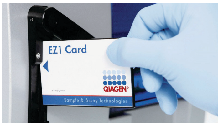
Figure 6. Ease of protocol setup using EZ1 DSP Cards. Inserting an EZ1 Card, preprogrammed with the protocol, into the EZ1 instrument.
