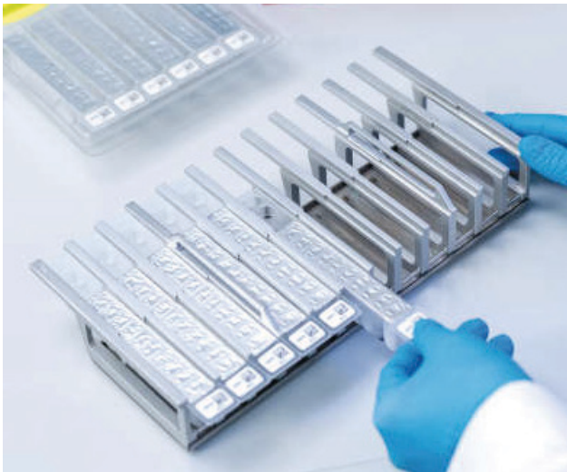
Figure 3. Reagent cartridge rack. The cartridge rack itself is labeled with an arrow to indicate the direction in which reagent cartridges (RCV) must be loaded.
