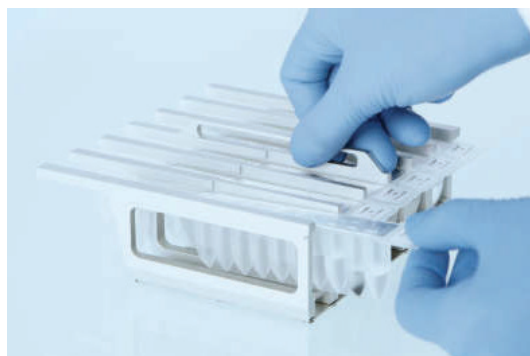
Figure 9. Loading the reagent cartridge rack. The cartridge rack itself is labeled with an arrow to indicate the direction in which reagent cartridges (RCV) must be loaded.
