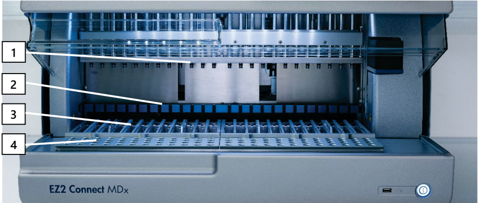
Figure 4. Overview of an EZ2 Connect MDx instrument. (1) Pipettor head, (2) magnet module, (3) cartridge rack, and (4) tip rack (labware holder).
