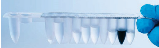
Figure 2. Reagent cartridge (RCV). Sealed, prefilled reagent cartridge (RCV) of the EZ1 DSP Virus Kit.
