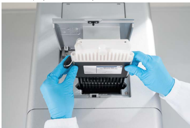
Figura 9. Instalarea QIAxcel Gel Cartridge.
