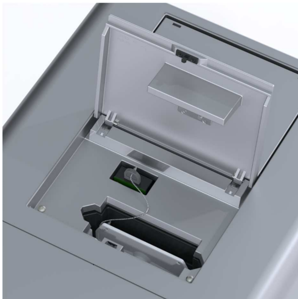
Figure 4. Installing the QIAxcel gel cartridge and smart key in the QIAxcel Connect instrument.
