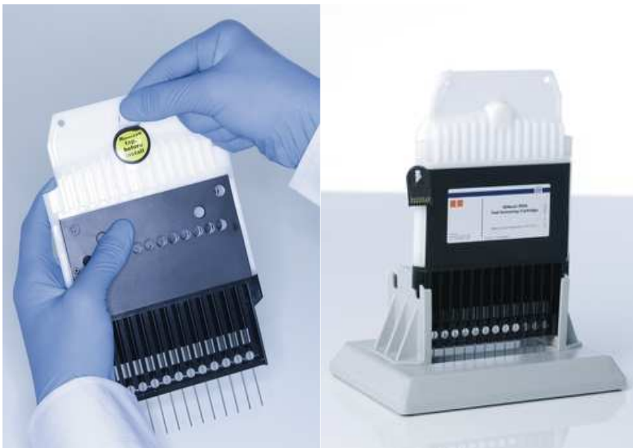
Figure 2. Preparing the QIAxcel gel cartridge. Upright storage in QX Cartridge Stand (cat. no. 929708) is recommended.
