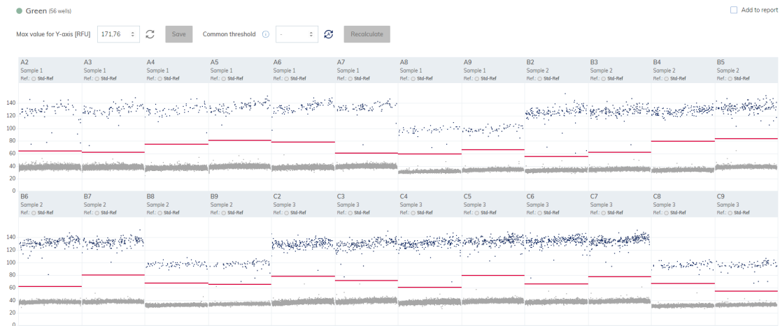
Example of 1D Scatterplot with enabled temperature gradient and 12 wells per row.
