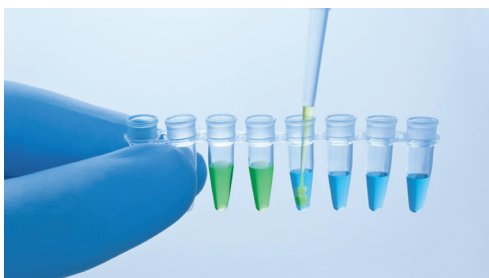
Figure 1. Accurate reaction set-up indicated by the built-in pipetting control. The master mix contains an inert blue dye, which when combined with the QuantiNova yellow template dilution buffer, turns the resulting solution green. This visual confirmation indicates that the reaction was set-up correctly.
