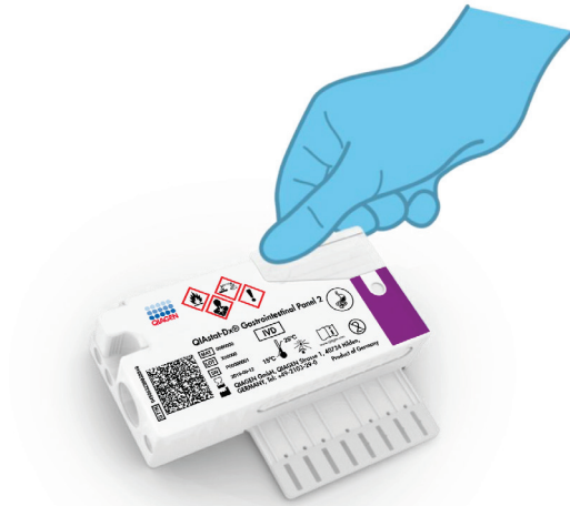
Figure 8. Closing the lid of the main port.
