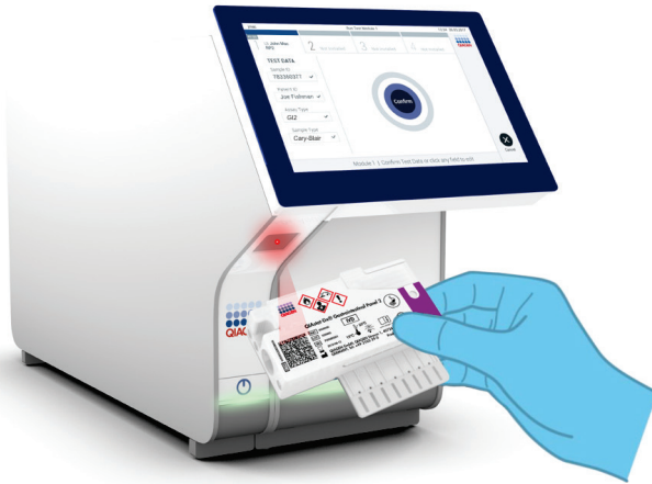
Figure 11. Scanning QIAstat-Dx Gastrointestinal Panel 2 Cartridge bar code.
