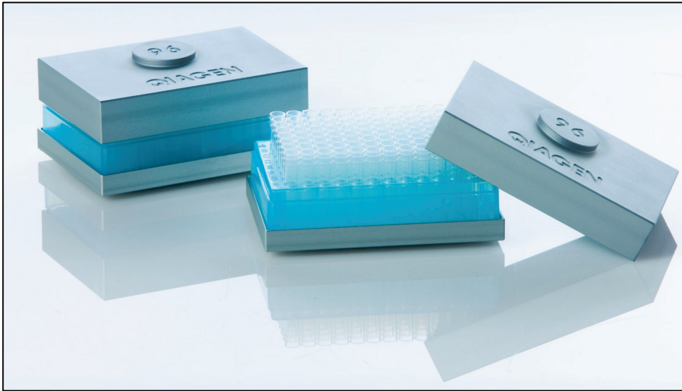
Figure 7. TissueLyser Adapter Set 2 x 96. Each adapter consists of a top plate and a bottom plate for holding a rack of capped collection microtubes.
