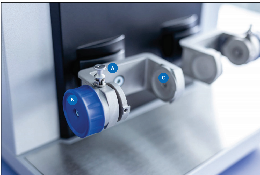
Figure 16. Left-hand clamp of the TissueLyser III. A Locking pin. B Handwheel. C Indentation in clamp.
