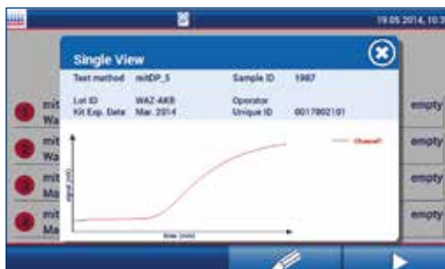
Figure 2. Real-time detection of isothermal amplification.
