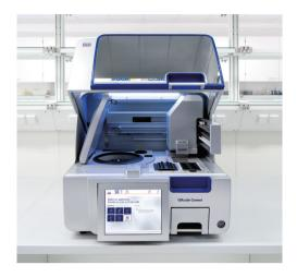
QIAcube Connect fully automates manual lyse\*, bind, wash and elution steps for up to 12 samples in a single run
