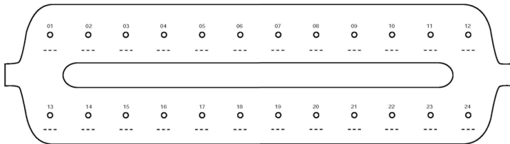
Figure 3. Labeling scheme for tubes and QIAamp UCP Mini Columns for use on the QIAvac 24 Plus vacuum system.
