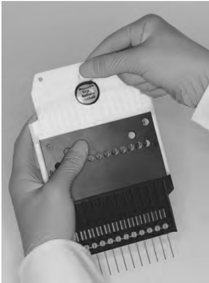
Figure 4. Preparing the QIAxcel Gel Cartridge.
