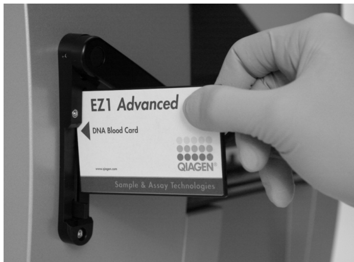
Figure 2. Ease of protocol setup using EZ1 Cards. Inserting an EZ1 Card, containing a protocol, into an EZ1 instrument. The instrument should only be switched on after an EZ1 Card is inserted. EZ1 Cards should not be exchanged while the instrument is switched on.
