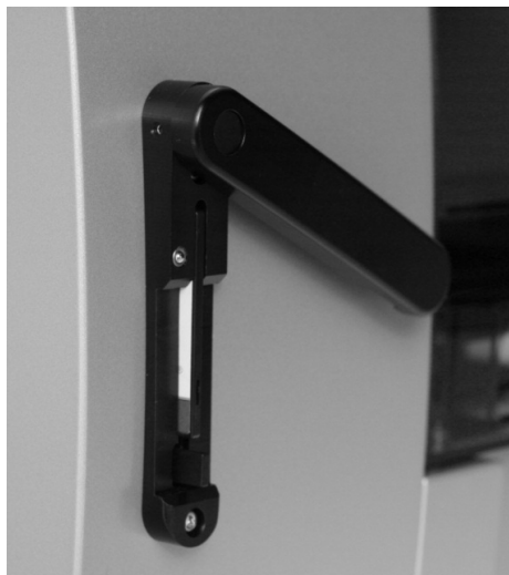
Figure 3. Complete insertion of EZ1 Card. The EZ1 Card must be completely inserted before the EZ1 instrument is switched on.
