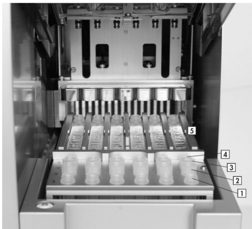
Figure 5. Typical EZ1 worktable. 1.) First row: In EZ1 RNA protocols, elution tubes (1.5 mL) are loaded here. 2.) Second row: In EZ1 RNA protocols, tip holders containing filter-tips loaded are loaded here. 3.) Third row: In EZ1 RNA protocols, tip holders containing filter-tips loaded are loaded here. 4.) Fourth row: In EZ1 RNA protocols, sample tubes (2 mL) are loaded here. 5.) Reagent cartridges loaded into the cartridge rack.
